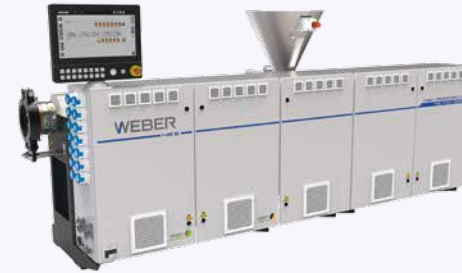
High Performance NE 40D Series for extrusion of polyolefin pipes Ø 10 - 1000 mm
